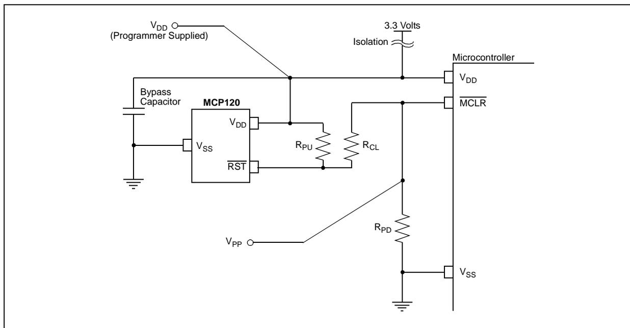
**FIGURE 2:** Active low open drain ICSP circuit.
