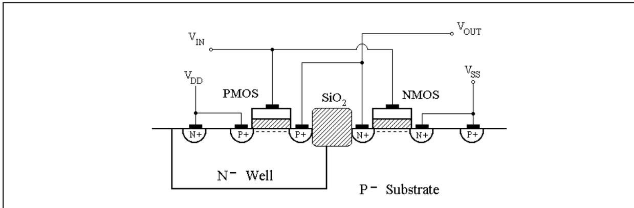
FIGURE 4: Push-Pull output in N-Well CMOS process.
